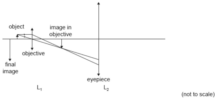
Two converging lenses are used to make an astronomical telescope. The focal length of the objective is 85.0 cm and that of the eyepiece is 2.50 cm. The telescope is used to form a final image of the Moon at infinity.
