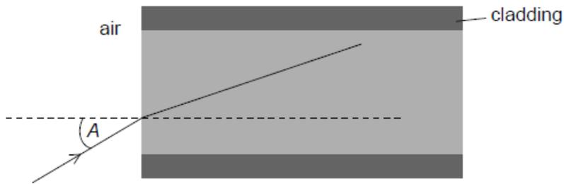
The ray makes an angle  $A$  with the normal at the air–core boundary. The refractive index of the core is 1.52 and that of the cladding is 1.48. Determine the largest angle  $A$  for which the light ray will stay within the core of the fibre.
