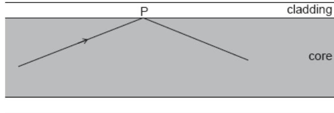
The refractive index of the core is 1.56 and that of the cladding is 1.34.
