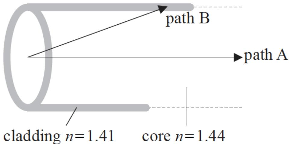
In a particular optic fibre of length  $2.00 \times 10^4$  m, the refractive index of the cladding is 1.41 and that of the core is 1.44.
