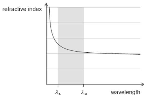
Two light rays enter the fibre at the same instant along the axes. Ray A has a wavelength of  $\lambda_A$  and ray B has a wavelength of  $\lambda_B$ . Discuss the effect that the difference in wavelength has on the rays as they pass along the fibre.
