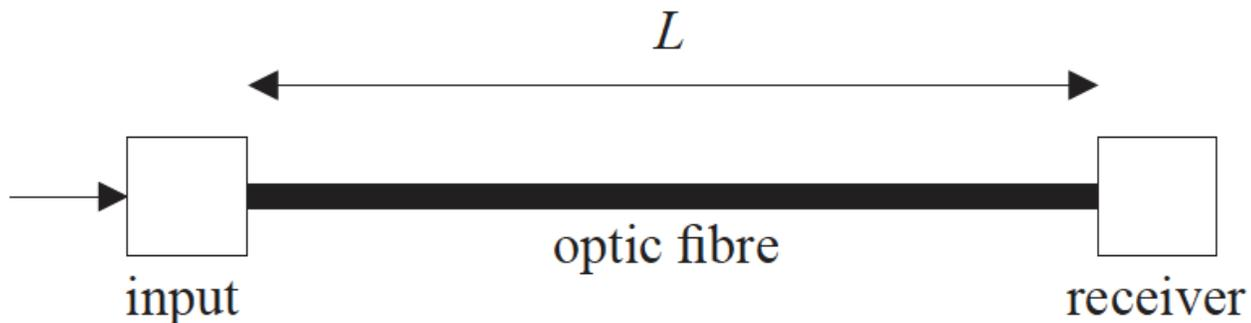
The noise power at the receiver is  $P_{\text{noise}} = 4.2 \mu\text{W}$ . The signal to noise ratio (*i. e.*  $10 \log \frac{P_{\text{signal}}}{P_{\text{noise}}}$ ) at the receiver must exceed 25 dB.
