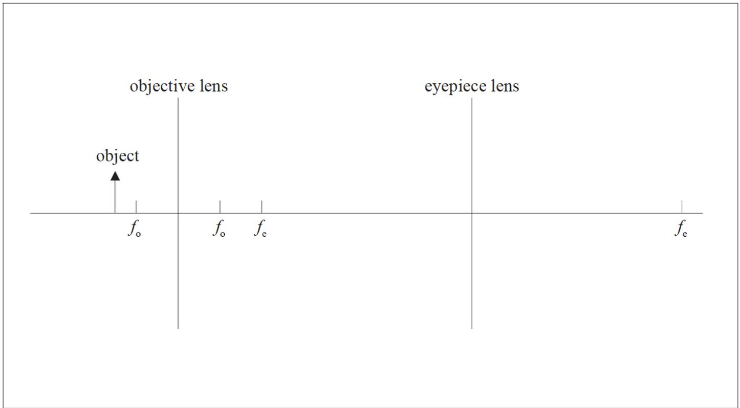
An object is placed 1.5 cm from the objective lens. The focal length  $f_o$  of the objective lens is 1.0 cm.
