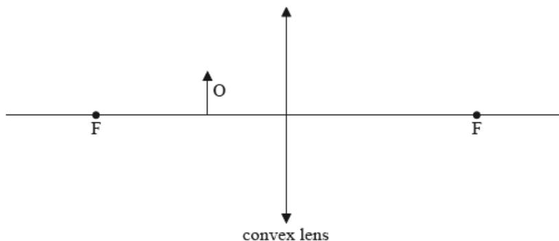
The position of the lens in (a) is changed so that a virtual image of the object is formed at the near point of the eye. The eye is very close to the lens.
