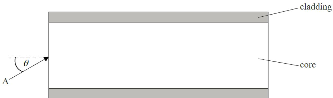
The refractive index of the core is 1.62 and the refractive index of the cladding is 1.52. The critical angle at the core-cladding boundary is  $70^\circ$ .
